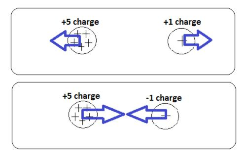
that students come to the conclusion that 1) Newton's third law applies to the electrostatic force like any other force. 2) the electric force weakens as the distance between the charges increase. This is sufficient to understand polarization forces.
