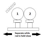
(3 points) Extra Credit: Two neutral conducting spheres on insulating stands are placed in contact. A negatively charged rod is then brought directly to the left of sphere **1**, but DOES NOT TOUCH either sphere. While the rod is held still, the sphere **2** is moved so that the spheres no longer touch. Then the charged rod is withdrawn.
